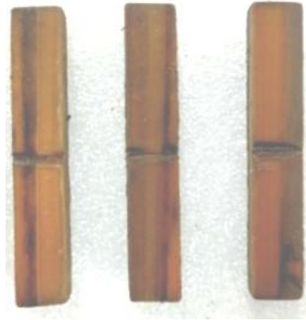
Fig. 12. Impact test specimens
