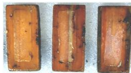
Fig. 9. Shrinkage test specimen
