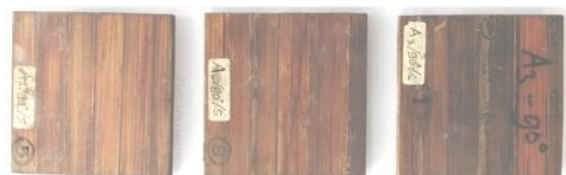
Fig. 8. Water content and density test specimens
