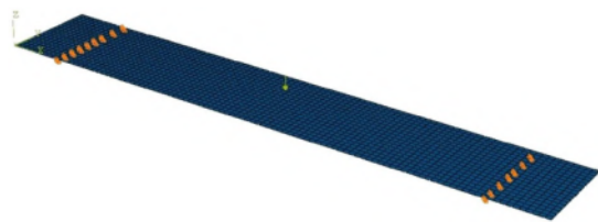
Figure 14: Bending test model for material model validation
