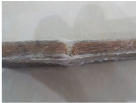
Figure 6: Fracture contour in tensile test specimen
