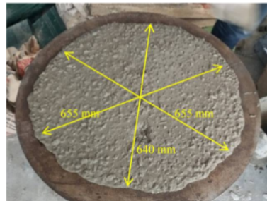
Fig. 2. SCC flowability measurement
