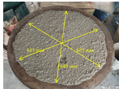
Fig. 2. SCC flowability measurement
