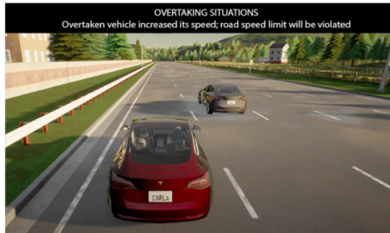
Fig. 6: The user interface for autopilot agent transparency based on the overtaking scenario
