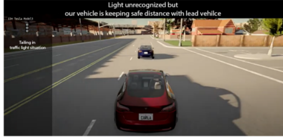
Fig. 4: The user interface for autopilot agent transparency based on TL situation scenario
