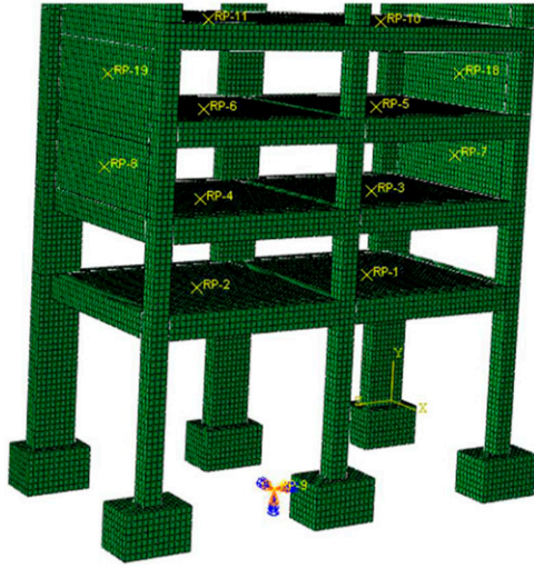
Figure 6. Boundary condition of the building model.
