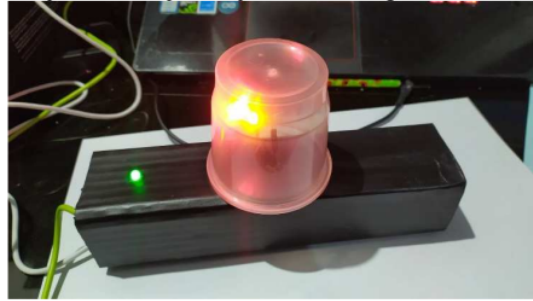
Fig. 4 The Library Noise Monitoring System’s Warning Sign
