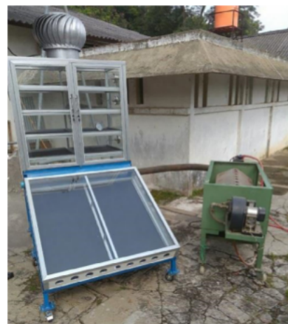
FIGURE 2 Hybrid solar dryer with blower and burner unit
