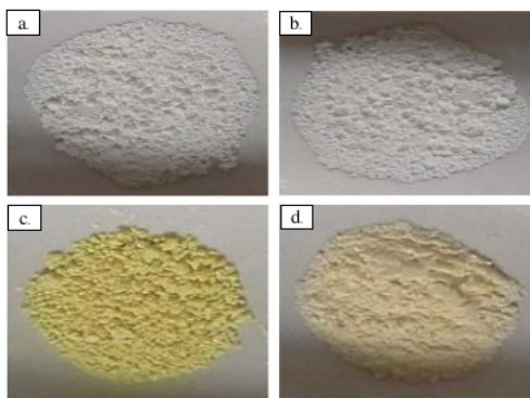
Figure 2. The products after drying in an oven for 24 hours at 110 °C, precipitated using (a) \text{NH}_4\text{OH} (BO1) or (b) \text{NaOH} (BO2); calcination of products (a) and (b) at 500 °C for 1 hour in a furnace generated (c) a bright yellow (BO3) and (d) yellow pale powder (BO4), respectively
