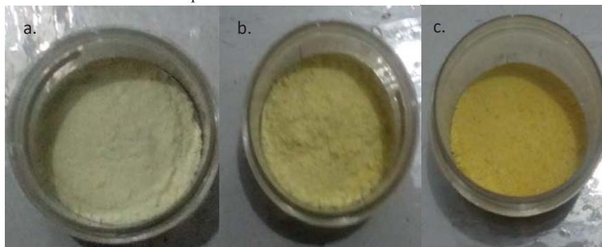
FIGURE 2. The result of bismuth oxide synthesis after calcination at: (a) 500^\circ\text{C} (b) 600^\circ\text{C} (c) 700^\circ\text{C}
