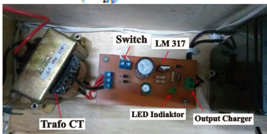
Fig. 5. Realization of Battery Charger Circuit using IC LM217
