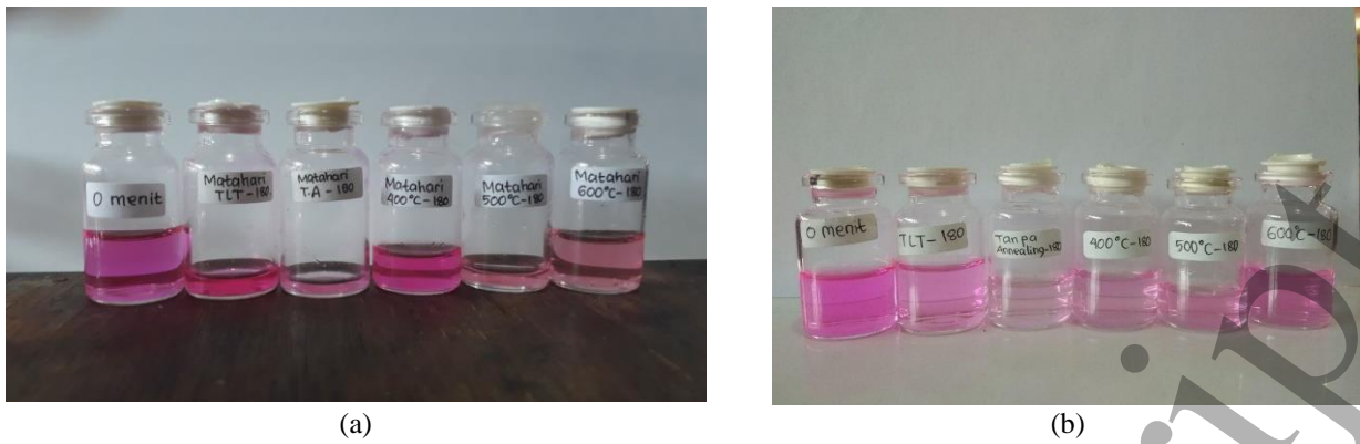
Figure 7. RhB solution after degradation below (a) sunlight (b) UV light lamp C
