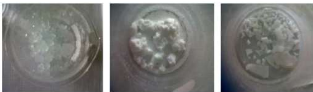
Figure 1. Silica gel (left), silica gel after heating at a temperature of 80 °C (middle) and xerogel product after heating at a temperature of 100 °C (right).
