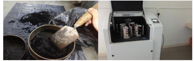
Figure 1. Filtering the baggase ash and High Energy Milling
