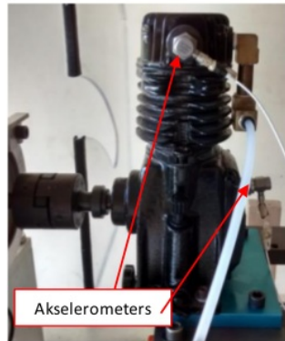
Figure 3. Accelerometer sensor location
