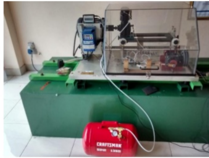
Figure 2. Reciprocating compressor setup on MFS
