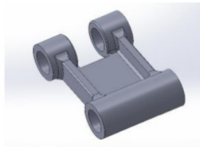
Figure 2: Design bucket link excavator
