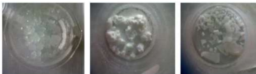
Figure 1. Silica gel (left), silica gel after heating at a temperature of 80 °C (middle) and xerogel product after heating at a temperature of 100 °C (right).
