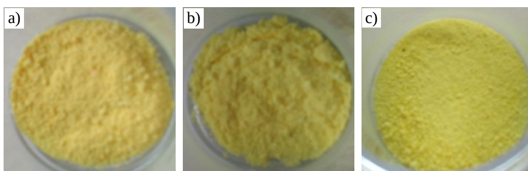
Figure 2 \text{Bi}_2\text{O}_3 synthesized using a) urea, b) glycine, and c) citric acid after calcination
