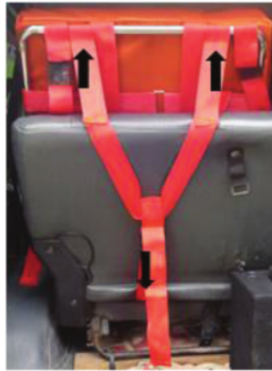
Figure 1. The installation of autistic mobile seat belt on a vehicle seat.
