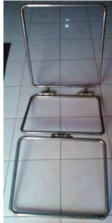
Figure 3. The frame of the autistic mobile seat.
