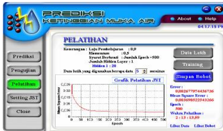
Figure 10. Display of the training results for model-1 with input are rainfall CH_{(Q)} s/d CH_{(t-24 \text{ hours})} and water level TMA_{(t)} s/d TMA_{(t-3 \text{ hours})}
