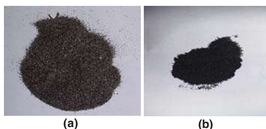
Fig. 1. The original iron sand from marina beach before extraction treatment with permanent magnet (A) Magnetite after extraction treatment
