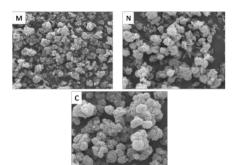
Figure 2. The SEM photographs at magnitude 20.000 x (M) synthesized zeolite/before modification, (H) Modified zeolite by NH<sub>4</sub>Cl, (C) Modified zeolite by NiCl<sub>2</sub>
