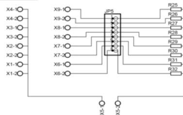
Gambar 6. Rangkain Pull Down
