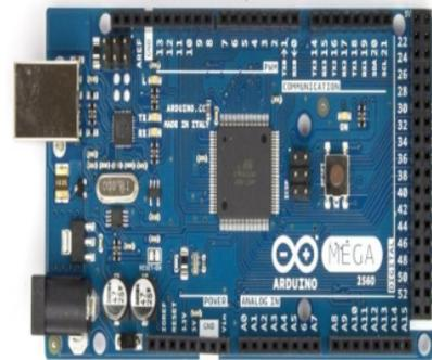
Gambar 1. Arduino Mega 2560
