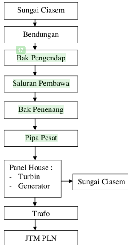
Gambar 1. Diagram Model Operasi PLTMH Cinta Mekar
