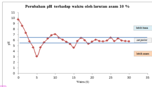
Fig. 4. Graph of changes in pH to time due to the addition of 10% acid solution
