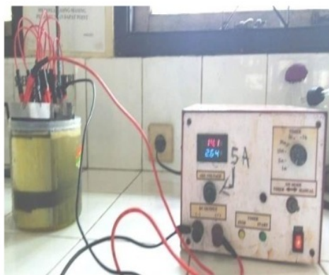
Figure 1. Electrocoagulation equipment of electroplating wastewater
