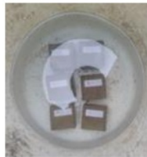
Figure 8. Soaking the mortar
