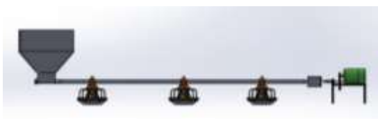
Fig. 2. Automatic chicken feed system
