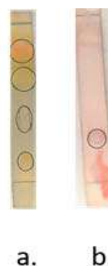
Fig. 3. TLC Profile of coconut PLs (a). Dragendorff stain (b). Ninhydrin stain
