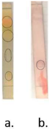
Fig 3. TLC Profile of coconut PLs (a). Dragendorff stain (b). Ninhydrin stain
