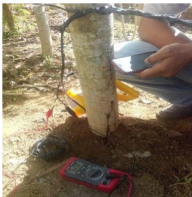
Figure 5. Photograph of potential measurement without load of the Galvanic cell using plant's sap.
