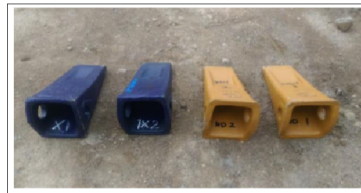
Figure-1. Excavator bucket teeth product; a) as-cast product (X1, X2), b) as-manufactured product (ND1, 2).
