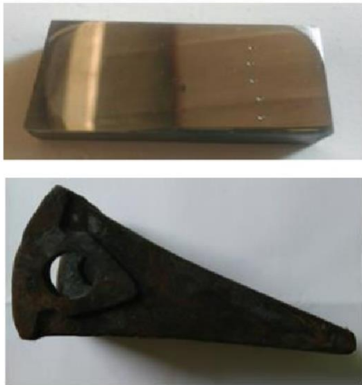
Figure-2. The bucket samples selected for measuring the hardness.
