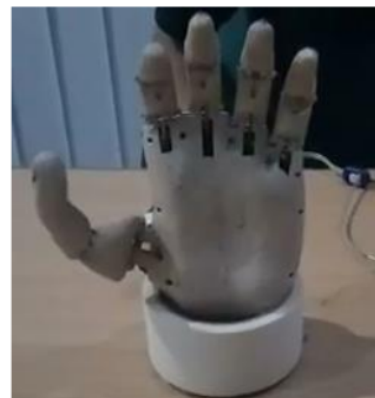
Figure 2. The final prototype of the proposed low-cost myoelectric hand
