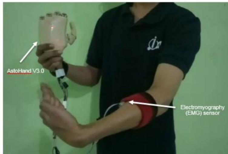
Figure 6. Electromyography sensor placement
