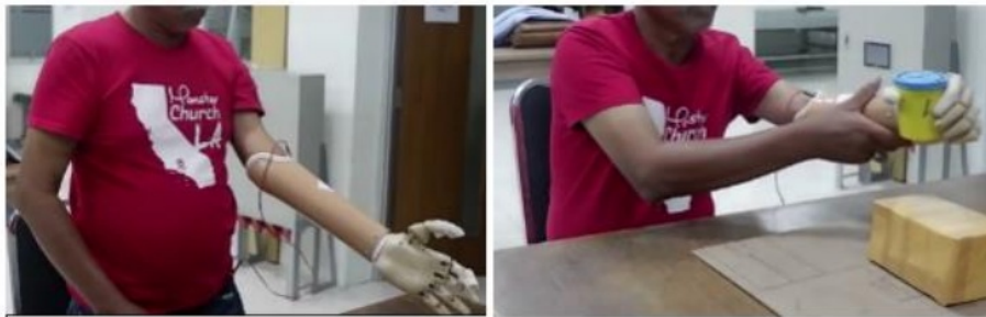
Figure 13. AstoHand V3.0 implemented on the study participant with transradial amputee
