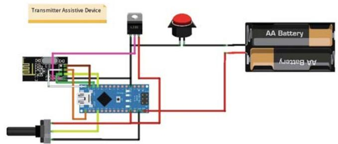
Fig. 3. Proposed transmitter hardware system
