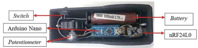
Fig. 4. The prototype of the transmitter hardware system (remote control)
