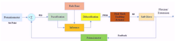
Figure 5. Fuzzy Logic control employed in the soft exoskeleton glove. Source: Authors
