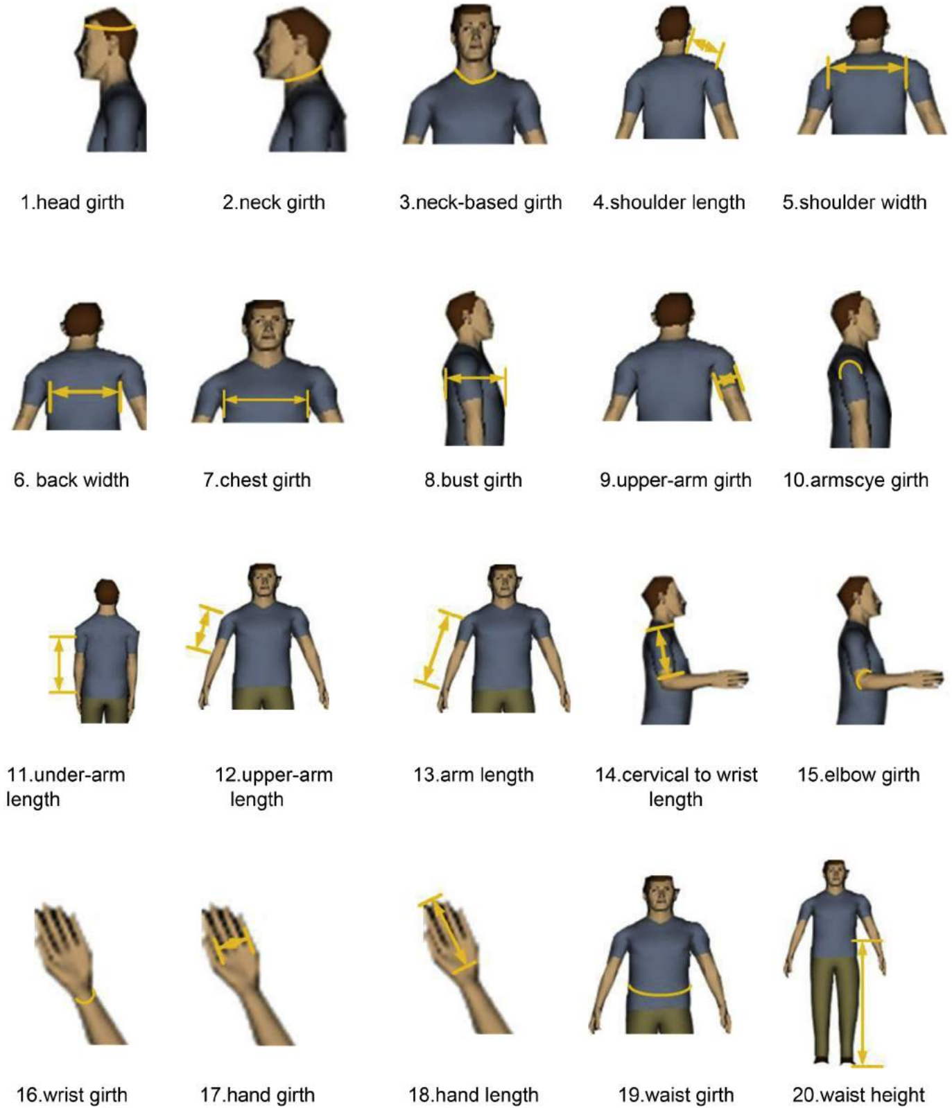
Fig. 1. Anthropometry dimensions for garment industries according to ISO 8559/1989.
