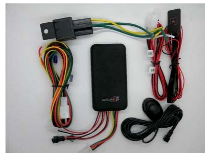
Fig. 2. GT06-A component which is equipped in truck.
