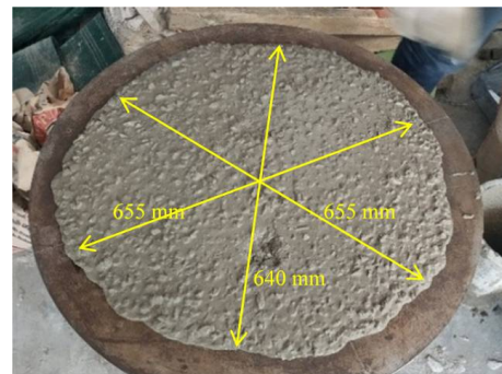
Fig. 2. SCC flowability measurement
