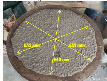
Fig. 2. SCC flowability measurement
