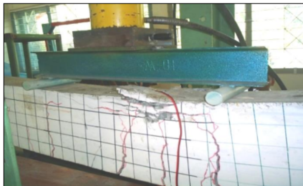
Figure 11. Normal beam failure under two points loads
