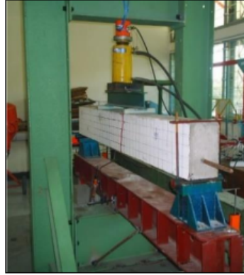
Figure 9. Experimental set-up for the normal beam and beam with CFRP
