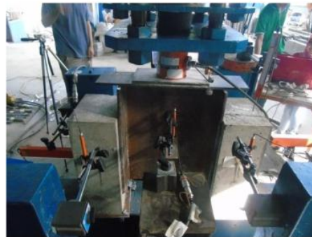
Gambar 3. Push-out test benda uji
