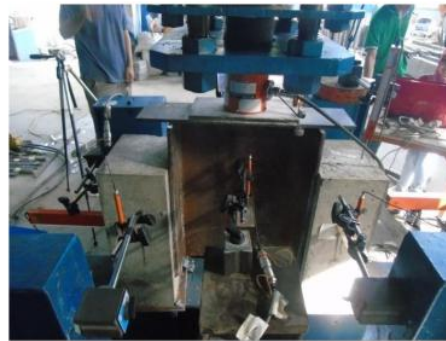
Gambar 3. Push-out test benda uji
