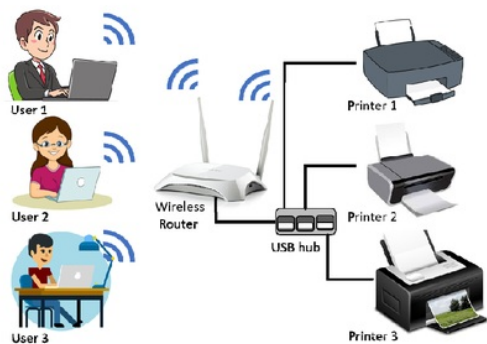
Fig. 1. The scenario of the proposed HT Wireless Printer Server system.
