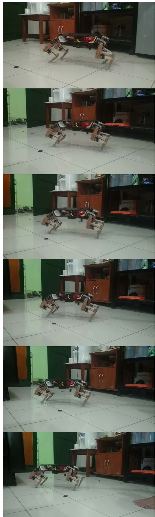
Fig. 8. Sequence images of the walking cat-like robot
