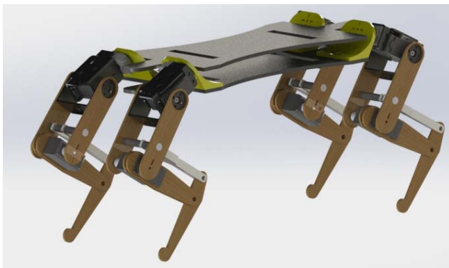
Fig. 1. 3D design of the cat-like robot.
