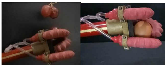
Fig. 11. Grasping test for delicate objects
