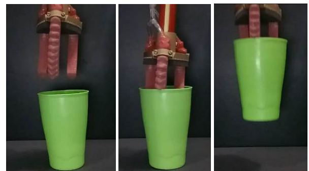
Fig. 10. Grasping an object using negative pressure
