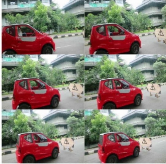
Fig. 10. Sequence images of automatic braking test
