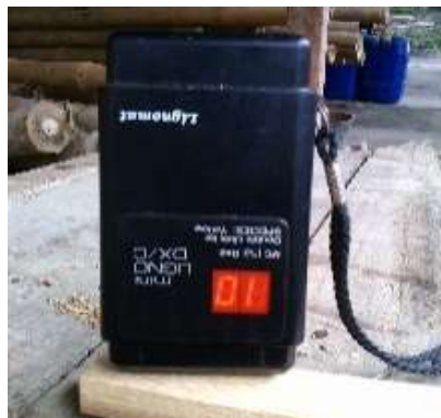
Figure 5 Calculation of MC using moisture meter
