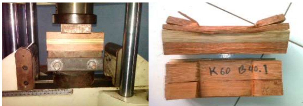
Gambar 9 Press tested and specimen tested
