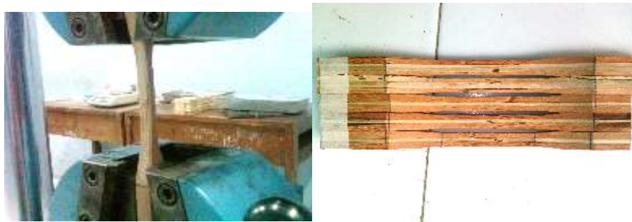
Figure 7 Process of tensile testing and the specimen after the test
