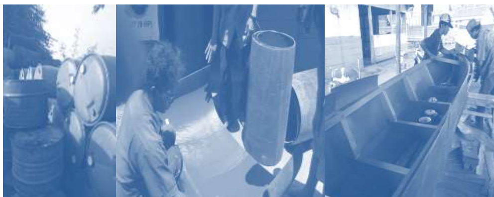
Figure 2 The use of HDPE plastic material used as a drum pack as a boat shell instead of wood.
