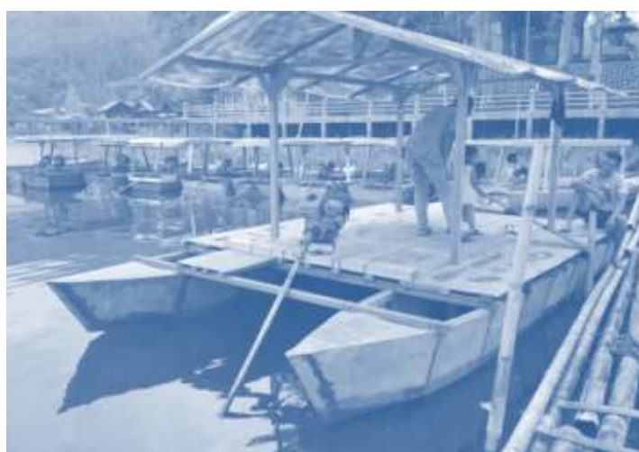
Figure 1 Catamaran Boat with Plastic HDPE which is used as a packaging drum produced by Kebondowo Banyubiru boat craftsmen.
