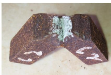
Figure 10. Fault of the 400 C Tempering Specimen
