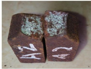
Figure 8. Quenching Specimen Fault
