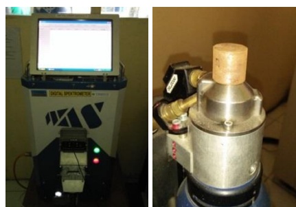
Figure 1. Spectrometer Testing Equipment and Test Specimens
