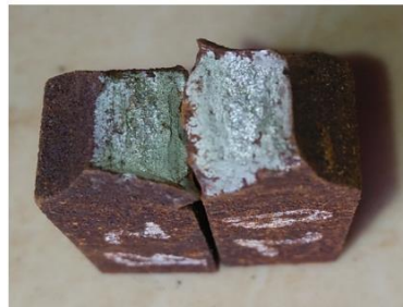
Figure 9. Fault of Tempering Specimen 200 °C
