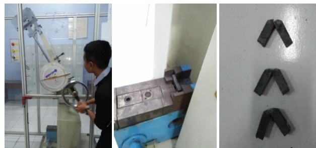
Figure 6. Impact testing process
