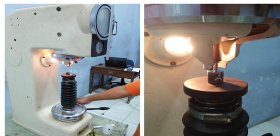
Figure 13. Hardness Testing Process Using the Vickers Method with a Load used of 40 kg
