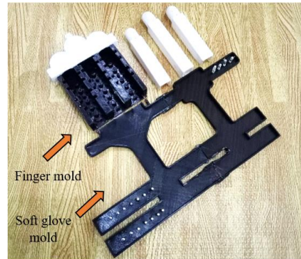
(c) Overall result of 3D printed mold design for exoskeleton glove. Fig. 2. 3D mold design of the proposed soft glove
