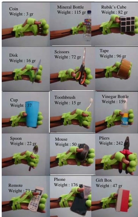
Fig. 16. The wearable glove provides mechanical support to the user's hand
