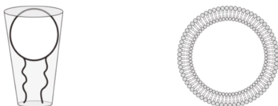
a. Molecular shape, Truncated cone b. Self-assembled shape, liposome
